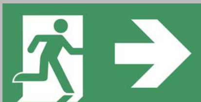
New escape sign according to DIN EN ISO 7010:2012-10 and ASR A1. 3:2013-02
