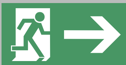
Previous escape sign according to DIN 4844-2:2001-02
