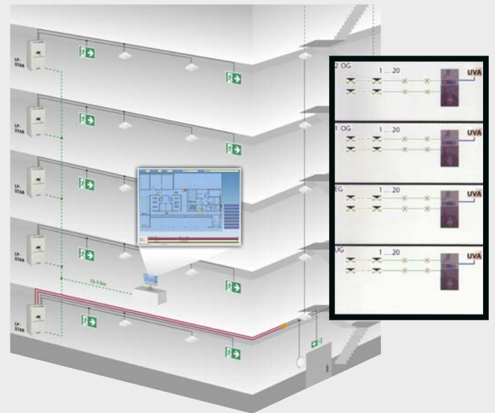
[39] Inter-fire compartment installation with central emergency power source (battery)
