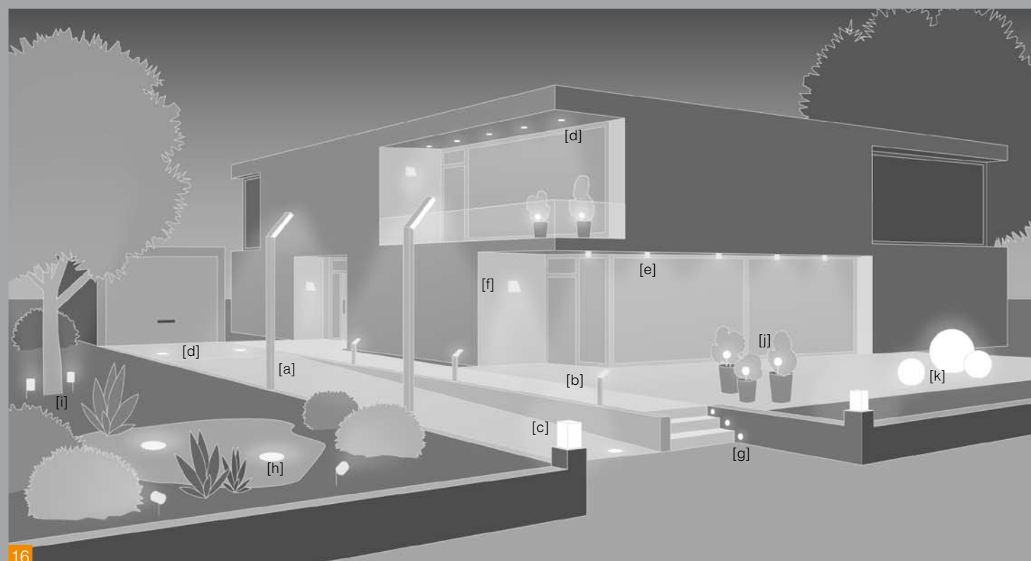
[16] Overview of luminaire types: [a] Column luminaires [b] Bollard luminaires [c] Pillar lights [d] Recessed luminaires (in-ground and recessed wall and ceiling luminaires) [e] Ceiling luminaires [f] Wall luminaires [g] Steplights [h] Underwater luminaires [i] Earth spike spots [j] Clamp luminaires [k] Light sculptures
